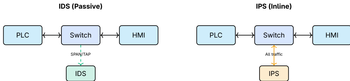
Figure 1: IDS (Passive) vs IPS (Inline) Deployment
